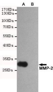
Western blot analysis of extracts from CHO-K1 (B) and CHO-K1 transfected by MMP-2 fragment(A) cell lysates using MMP-2 mouse mAb (1:2000 diluted) .Predicted band size:30KDa. Observed band size:30KDa.
